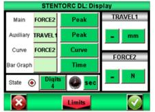
Configure the measuring screen in order to display the peak force on the main display area and the peak deflection value on the auxiliary display area:
