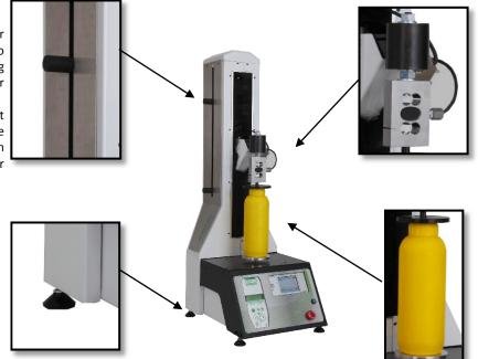
Installing the load cell:
